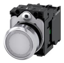
Illuminated pushbutton, 22 mm, round, metal, shiny, white, pushbutton, flat, momentary contact type, with holder, 1NO, LED module with integrated LED 24 V AC/DC, screw terminal, with laser labeling, upper case and lower case, Always upper case at the beginning of the word
