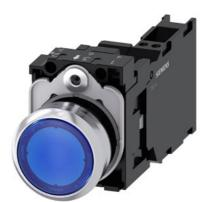
Illuminated pushbutton, 22 mm, round, metal, shiny, blue, pushbutton, flat, momentary contact type, with holder, 1 NO+1 NC, LED module with integrated LED 24 V AC/DC, spring-type terminal, with laser labeling, inscription or symbol Customer-specific selection with SIRIUS ACT configurator (CIN)
