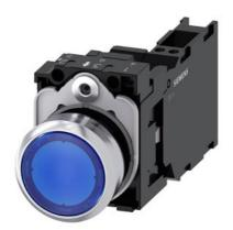
Illuminated pushbutton, 22 mm, round, metal, shiny, blue, pushbutton, flat, momentary contact type, with holder, 1 NO+1 NC, LED module with integrated LED 24 V AC/DC, spring-type terminal, with laser labeling, lower case
