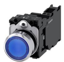
Illuminated pushbutton, 22 mm, round, metal, shiny, blue, pushbutton, flat, momentary contact type, with holder, 1 NO+1 NC, LED module with integrated LED 24 V AC/DC, spring-type terminal, with laser labeling, upper case
