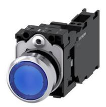
Illuminated pushbutton, 22 mm, round, metal, shiny, blue, pushbutton, flat, momentary contact type, with holder, 1 NO+1 NC, LED module with integrated LED 24 V AC/DC, spring-type terminal, with laser labeling, upper case and lower case, always upper case at beginning of line
