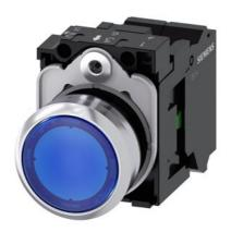
Illuminated pushbutton, 22 mm, round, metal, shiny, blue, pushbutton, flat, momentary contact type, with holder, 1NO, LED module with integrated LED 24 V AC/DC, spring-type terminal, with laser labeling, inscription or symbol Customerspecific selection with SIRIUS ACT configurator (CIN)
