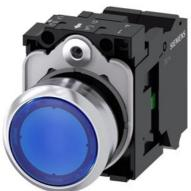
Illuminated pushbutton, 22 mm, round, metal, shiny, blue, pushbutton, flat, momentary contact type, with holder, 1NO, LED module with integrated LED 24 V AC/DC, spring-type terminal, with laser labeling, upper case and lower case, Always upper case at the beginning of the word
