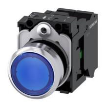
Illuminated pushbutton, 22 mm, round, metal, shiny, blue, pushbutton, flat, momentary contact type, with holder, 1NO, LED module with integrated LED 24 V AC/DC, spring-type terminal, with laser labeling, symbol number according to, ISO 7000 or IEC 60417
