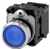
Illuminated pushbutton, 22 mm, round, metal, shiny, blue, pushbutton, flat, momentary contact type, with holder, 1NO, LED module with integrated LED 24 V AC/DC, spring-type terminal, with laser labeling, upper case and lower case, always upper case at beginning of line
