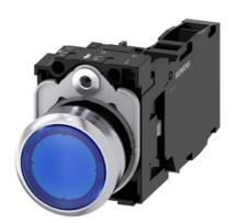
Illuminated pushbutton, 22 mm, round, metal, shiny, blue, pushbutton, flat, momentary contact type, with holder, 1 NO+1 NC, LED module with integrated LED 24 V AC/DC, screw terminal, with laser labeling, inscription or symbol Customer-specific selection with SIRIUS ACT configurator (CIN)
