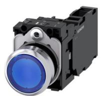
Illuminated pushbutton, 22 mm, round, metal, shiny, blue, pushbutton, flat, momentary contact type, with holder, 1 NO+1 NC, LED module with integrated LED 24 V AC/DC, screw terminal, with laser labeling, upper case and lower case, Always upper case at the beginning of the word
