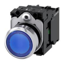
Illuminated pushbutton, 22 mm, round, metal, shiny, blue, pushbutton, flat, momentary contact type, with holder, 1NO, LED module with integrated LED 24 V AC/DC, screw terminal, with laser labeling, upper case
