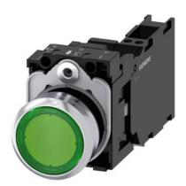
Illuminated pushbutton, 22 mm, round, metal, shiny, green, pushbutton, flat, momentary contact type, with holder, 1 NO+1 NC, LED module with integrated LED 24 V AC/DC, spring-type terminal, with laser labeling, inscription or symbol Customer-specific selection with SIRIUS ACT configurator (CIN)
