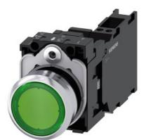
Illuminated pushbutton, 22 mm, round, metal, shiny, green, pushbutton, flat, momentary contact type, with holder, 1 NO+1 NC, LED module with integrated LED 24 V AC/DC, spring-type terminal, with laser labeling, upper case and lower case, Always upper case at the beginning of the word
