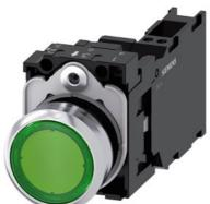
Illuminated pushbutton, 22 mm, round, metal, shiny, green, pushbutton, flat, momentary contact type, with holder, 1 NO+1 NC, LED module with integrated LED 24 V AC/DC, spring-type terminal, with laser labeling, symbol number according to, ISO 7000 or IEC 60417
