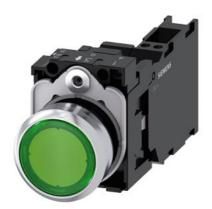
Illuminated pushbutton, 22 mm, round, metal, shiny, green, pushbutton, flat, momentary contact type, with holder, 1 NO+1 NC, LED module with integrated LED 24 V AC/DC, spring-type terminal, with laser labeling, upper case and lower case, always upper case at beginning of line
