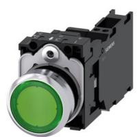
Illuminated pushbutton, 22 mm, round, metal, shiny, green, pushbutton, flat, momentary contact type, with holder, 1 NO+1 NC, LED module with integrated LED 24 V AC/DC, spring-type terminal, Z=20-unit packaging
