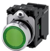
Illuminated pushbutton, 22 mm, round, metal, shiny, green, pushbutton, flat, momentary contact type, with holder, 1NO, LED module with integrated LED 24 V AC/DC, spring-type terminal, with laser labeling, inscription or symbol Customer-specific selection with SIRIUS ACT configurator (CIN)
