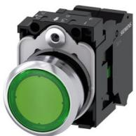
Illuminated pushbutton, 22 mm, round, metal, shiny, green, pushbutton, flat, momentary contact type, with holder, 1NO, LED module with integrated LED 24 V AC/DC, spring-type terminal, with laser labeling, upper case and lower case, always upper case at beginning of line
