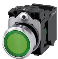
Illuminated pushbutton, 22 mm, round, metal, shiny, green, pushbutton, flat, momentary contact type, with holder, 1NO, LED module with integrated LED 24 V AC/DC, spring-type terminal, Z=20-unit packaging
