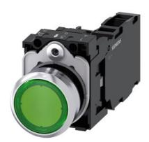
Illuminated pushbutton, 22 mm, round, metal, shiny, green, pushbutton, flat, momentary contact type, with holder, 1 NO+1 NC, LED module with integrated LED 24 V AC/DC, screw terminal, with laser labeling, symbol number according to, ISO 7000 or IEC 60417
