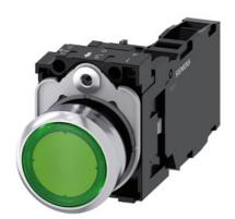
Illuminated pushbutton, 22 mm, round, metal, shiny, green, pushbutton, flat, momentary contact type, with holder, 1 NO+1 NC, LED module with integrated LED 24 V AC/DC, screw terminal, with laser labeling, lower case
