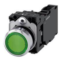
Illuminated pushbutton, 22 mm, round, metal, shiny, green, pushbutton, flat, momentary contact type, with holder, 1 NO+1 NC, LED module with integrated LED 24 V AC/DC, screw terminal, with laser labeling, upper case and lower case, always upper case at beginning of line
