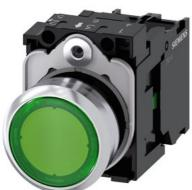
Illuminated pushbutton, 22 mm, round, metal, shiny, green, pushbutton, flat, momentary contact type, with holder, 1 NO, LED module with integrated LED 24 V AC/DC, screw terminal
