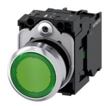
Illuminated pushbutton, 22 mm, round, metal, shiny, green, pushbutton, flat, momentary contact type, with holder, 1NO, LED module with integrated LED 24 V AC/DC, screw terminal, with laser labeling, symbol number according to, ISO 7000 or IFC 60417
