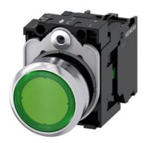
Illuminated pushbutton, 22 mm, round, metal, shiny, green, pushbutton, flat, momentary contact type, with holder, 1NO, LED module with integrated LED 24 V AC/DC, screw terminal, Z=20-unit packaging
