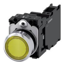
Illuminated pushbutton, 22 mm, round, metal, shiny, yellow, pushbutton, flat, momentary contact type, with holder, 1 NO+1 NC, LED module with integrated LED 24 V AC/DC, spring-type terminal, with laser labeling, inscription or symbol Customer-specific selection with SIRIUS ACT configurator (CIN)
