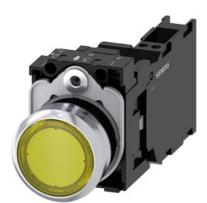
Illuminated pushbutton, 22 mm, round, metal, shiny, yellow, pushbutton, flat, momentary contact type, with holder, 1 NO+1 NC, LED module with integrated LED 24 V AC/DC, spring-type terminal, with laser labeling, lower case
