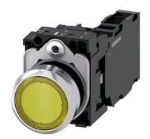
Illuminated pushbutton, 22 mm, round, metal, shiny, yellow, pushbutton, flat, momentary contact type, with holder, 1 NO+1 NC, LED module with integrated LED 24 V AC/DC, screw terminal, with laser labeling, lower case
