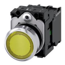
Illuminated pushbutton, 22 mm, round, metal, shiny, yellow, pushbutton, flat, momentary contact type, with holder, 1NO, LED module with integrated LED 24 V AC/DC, screw terminal, with laser labeling, inscription or symbol Customer-specific selection with SIRIUS ACT configurator (CIN)
