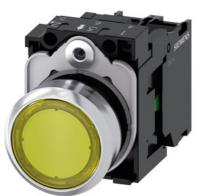
Illuminated pushbutton, 22 mm, round, metal, shiny, yellow, pushbutton, flat, momentary contact type, with holder, 1NO, LED module with integrated LED 24 V AC/DC, screw terminal, with laser labeling, upper case and lower case, Always upper case at the beginning of the word
