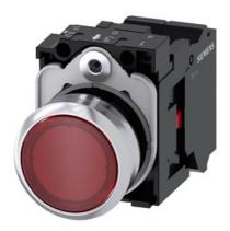
Illuminated pushbutton, 22 mm, round, metal, shiny, red, pushbutton, flat, momentary contact type, with holder, 1NC, LED module with integrated LED 24 V AC/DC, spring-type terminal, with laser labeling, inscription or symbol Customerspecific selection with SIRIUS ACT configurator (CIN)
