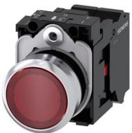
Illuminated pushbutton, 22 mm, round, metal, shiny, red, pushbutton, flat, momentary contact type, with holder, 1NC, LED module with integrated LED 24 V AC/DC, spring-type terminal, with laser labeling, upper case and lower case, Always upper case at the beginning of the word
