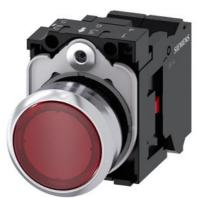
Illuminated pushbutton, 22 mm, round, metal, shiny, red, pushbutton, flat, momentary contact type, with holder, 1NC, LED module with integrated LED 24 V AC/DC, spring-type terminal, with laser labeling, upper case
