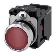
Illuminated pushbutton, 22 mm, round, metal, shiny, red, pushbutton, flat, momentary contact type, with holder, 1NC, LED module with integrated LED 24 V AC/DC, spring-type terminal, with laser labeling, upper case and lower case, always upper case at beginning of line
