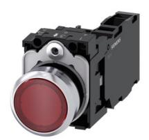
Illuminated pushbutton, 22 mm, round, metal, shiny, red, pushbutton, flat, momentary contact type, with holder, 1 NO+1 NC, LED module with integrated LED 24 V AC/DC, screw terminal, with laser labeling, upper case
