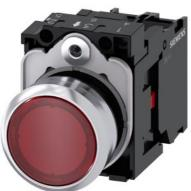
Illuminated pushbutton, 22 mm, round, metal, shiny, red, pushbutton, flat, momentary contact type, with holder, 1NC, LED module with integrated LED 24 V AC/DC, screw terminal, with laser labeling, inscription or symbol Customer-specific selection with SIRIUS ACT configurator (CIN)
