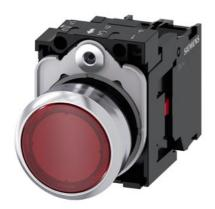
Illuminated pushbutton, 22 mm, round, metal, shiny, red, pushbutton, flat, momentary contact type, with holder, 1NC, LED module with integrated LED 24 V AC/DC, screw terminal, with laser labeling, symbol number according to, ISO 7000 or IFC 60417
