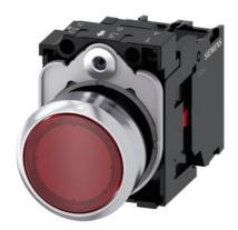
Illuminated pushbutton, 22 mm, round, metal, shiny, red, pushbutton, flat, momentary contact type, with holder, 1NC, LED module with integrated LED 24 V AC/DC, screw terminal, with laser labeling, lower case
