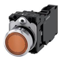
Illuminated pushbutton, 22 mm, round, metal, shiny, amber, pushbutton, flat, momentary contact type, with holder, 1 NO+1 NC, LED module with integrated LED 24 V AC/DC, screw terminal, with laser labeling, inscription or symbol Customer-specific selection with SIRIUS ACT configurator (CIN)
