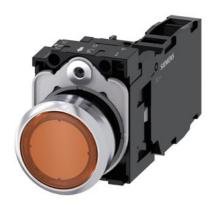
Illuminated pushbutton, 22 mm, round, metal, shiny, amber, pushbutton, flat, momentary contact type, with holder, 1 NO+1 NC, LED module with integrated LED 24 V AC/DC, screw terminal, with laser labeling, symbol number according to, ISO 7000 or IEC 60417
