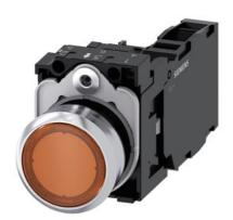
Illuminated pushbutton, 22 mm, round, metal, shiny, amber, pushbutton, flat, momentary contact type, with holder, 1 NO+1 NC, LED module with integrated LED 24 V AC/DC, screw terminal, with laser labeling, lower case
