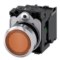
Illuminated pushbutton, 22 mm, round, metal, shiny, amber, pushbutton, flat, momentary contact type, with holder, 1NO, LED module with integrated LED 24 V AC/DC, screw terminal, Z=20-unit packaging
