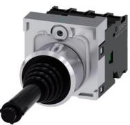
Coordinate switch, 22 mm, round, metal shiny, black, 4 switch positions, latching, with mechanical interlocking, in O position, with holder, 1 NO, 1 NO, 1 NO, 1 NO, screw terminal, Z=20-unit packaging
