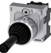
Coordinate switch, 22 mm, round, metal shiny, black, 2 switch positions, vertical latching, with mechanical interlocking, in O position, with holder, 1 NO, 1 NO, screw terminal, Z=20-unit packaging
