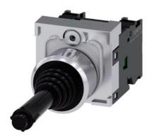
Coordinate switch, 22 mm, round, metal shiny, black, 2 switch positions, horizontal latching, with mechanical interlocking, in O position, with holder, 1 NO, 1 NO, screw terminal, Z=20-unit packaging
