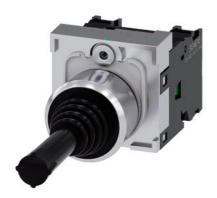
Coordinate switch, 22 mm, round, metal shiny, black, 2 switch positions, horizontal latching, without mechanical interlocking, in O position, with holder, 1 NO, 1 NO, screw terminal,
