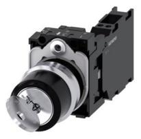
RONIS key-operated switch, 22 mm, round, metal, shiny, lock number SB30, with 2 keys, 2 switch positions O-I, latching, actuating angle 90°, 10:30h/13:30h, key removal O+I, with holder, 1 NO+1 NC, spring-type terminal, possible special locks: SB31, 421, 455 inscription or symbol Customer-specific selection with SIRIUS ACT configurator (CIN)
