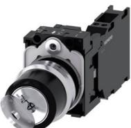
RONIS key-operated switch, 22 mm, round, metal, shiny, lock number SB30, with 2 keys, 2 switch positions O-I, latching, actuating angle 90°, 10:30h/13:30h, key removal O+I, with holder, 1 NO+1 NC, spring-type terminal, possible special locks: SB31, 421, 455, upper case
