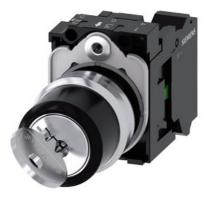
RONIS key-operated switch, 22 mm, round, metal, shiny, lock number SB30, with 2 keys, 2 switch positions O-I, latching, actuating angle 90°, 10:30h/13:30h, key removal O+I, with holder, 1 NO, spring-type terminal, possible special locks: SB31, 421, 455
